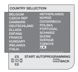
Select the country by using **Up/Down**, **Left/Right**movement buttons and press **OK** button to start the auto programming. **Channel Search**menu will be displayed and digital channels are scanned and stored in the memory.
